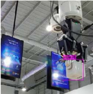
4. Checks the object existence by using the second camera (YOLO v3).
